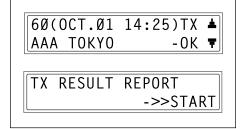
To print the transmission result report, press the [Start] key. After the transmission result report is printed, the main screen appears.
